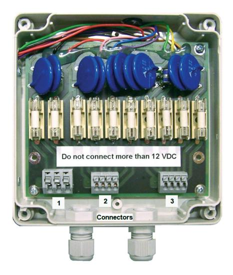
There is a push button between connector 2 pin 4 and connector 3 pin 3 mounted to configure the display; see chapter 3.
