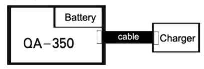
Charging method: the charger cable connects the host to the charger, which can achieve the battery charging. The charging time is about 1.5-3 hours. When all indicating lights on the charger turn from red to blue, it indicates the completion of charging (Two lights is red When Charging).
