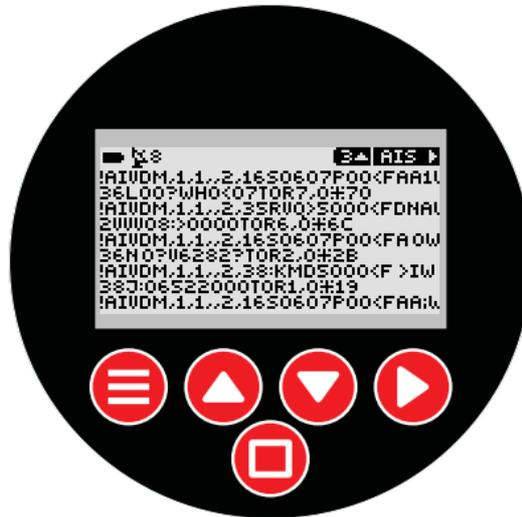
The decode history sub screen provides a means to view time-stamped entries, and also allows the entries to be selected to used with the direction finding screen (see Target Setting). Only AIS-SART messages are listed in the history.
