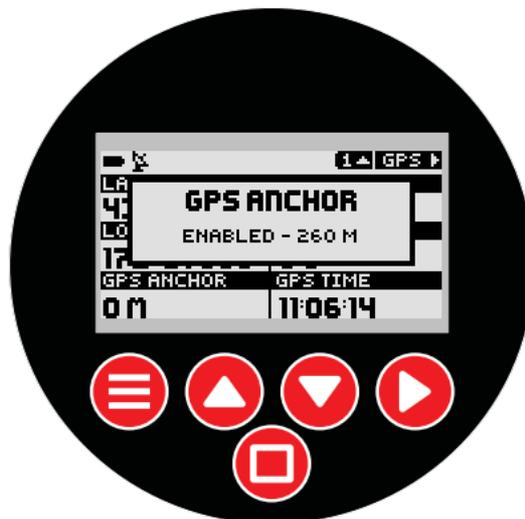
Pressing the square button again will unset the GPS anchor, and allow a new position to be set when the square button is pressed again.
