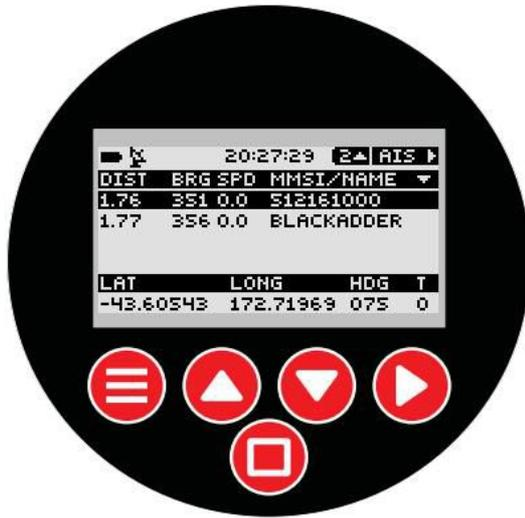
The SART (Search and Rescue Transponder) screen provides information relating to AIS distress type transmitters operating on both 161.975MHz and 162.025MHz. These transponders are commonly used as man-overboard transmitters.
