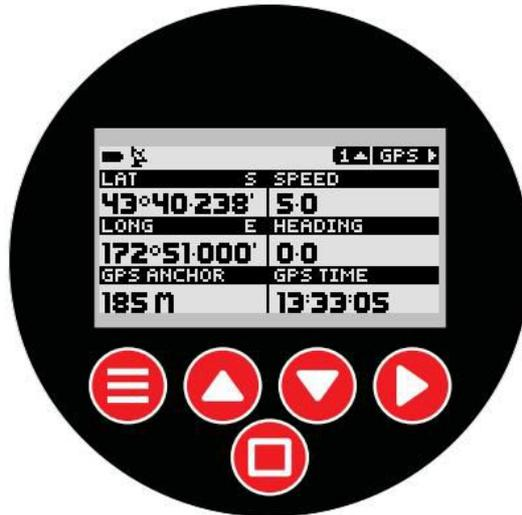
The GPS raw data sub screen provides real time updates of provided GPGLA and GPRMC NMEA sentences that are used to determine the current location, quality of fix and time.
