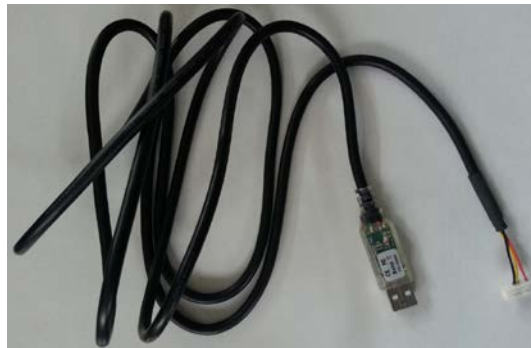
Fig. 73 Example of USB⇄COM(TTL1.8V) conversion cable
