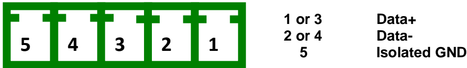
Fig. 44 COM1 Connector pin assignment
