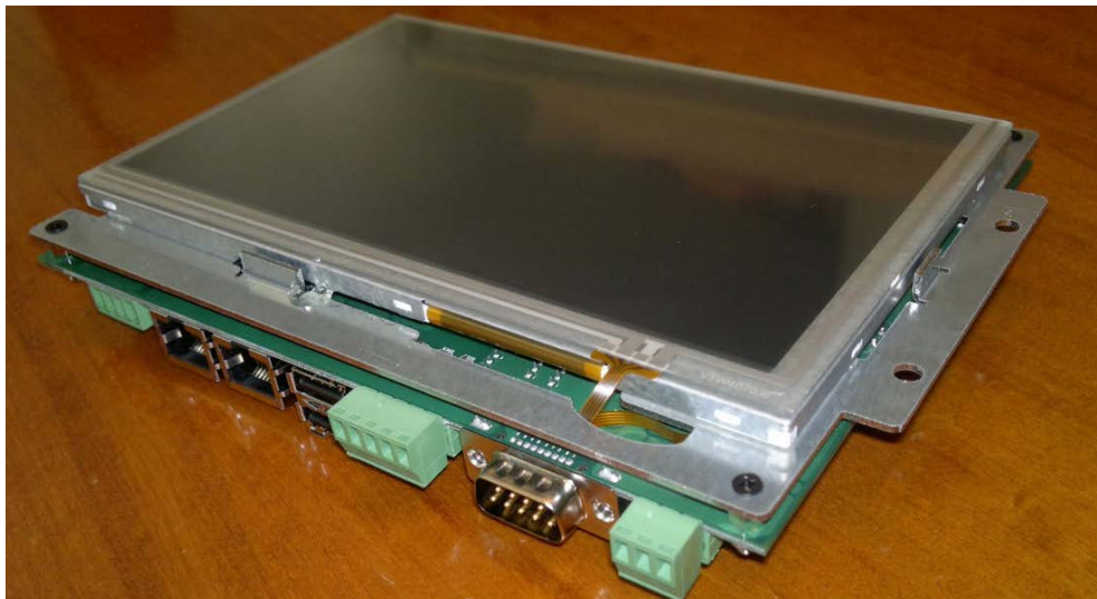
Fig. 93 The 7" LCD and the C2 assembled together
