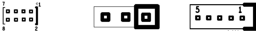
Fig. 5 Examples of Silk-Screen figures to recognize Pin 1
