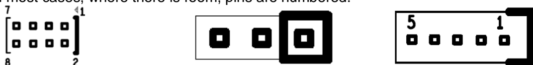
Fig. 33 Examples of Silk-Screen figures to recognize Pin 1
