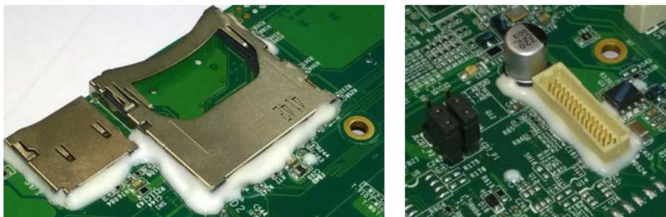
Fig. 103 Coating Protection for uSD/SD (left) and LVDS LCD (right) connectors
