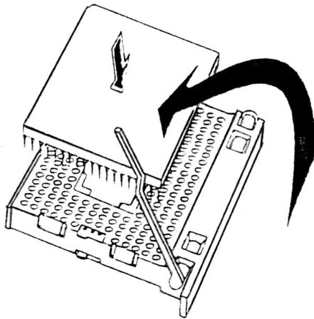
Figure 3-3 Removing CPU
