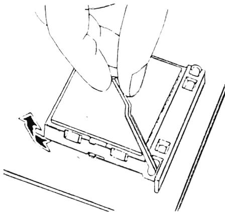
Figure 3-4 Installing CPU
