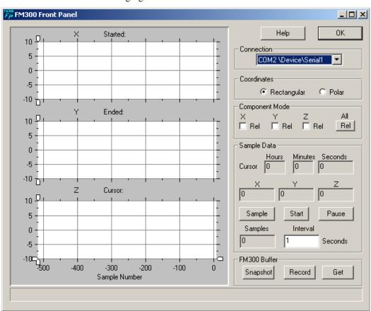
Once communication has been established with the FVM400, the FVM400 is set to the default mode, Rectangular coordinate system and Absolute measurement mode, and the controls are enabled as shown in the following figure.
