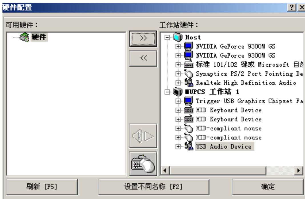
Now the “USB Audio Device” goes to MUPCS Station 1, and the audio card set up to use for Station 1 alone.
