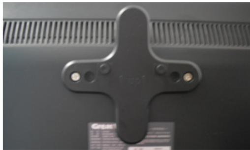
2. Put the station box to the bracket, sliding it down will be ok, no need other screws.
