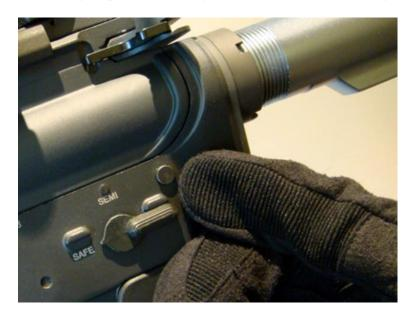
Then pull it from the other side until you hear a click. Once you hear a click, the receiver will immediately open. Please do not use any sharp or hard object as this might scratch the surface of the receiver.
