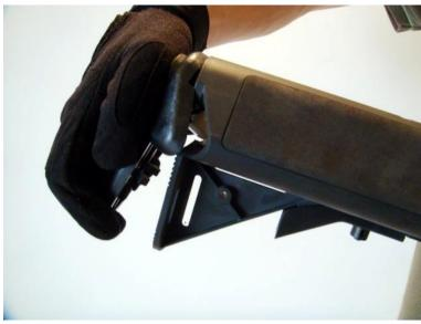
After the cover is removed, push the battery into the stock and slightly pull the wire **outward** to facilitate the position of the internal wiring.
