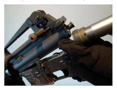
To take the cylinder unit out, pull back the charging handle along with the latch on its left side. The cylinder unit will slide along with the charging handle.
