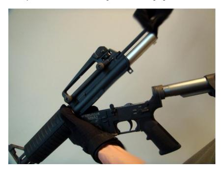
After the cylinder unit is removed, the charging handle can also be taken out by pulling it out all the way and then tilt it upward. To remove the inner barrel, use a plastic rod and insert it from the muzzle end. Run the rod along the inner wall of the outer barrel until it touches the tip of the inner barrel, then push the inner barrel out.
