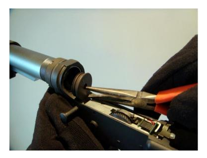
After gaining access to the circuit board and the fuse, gently remove the fuse from its socket using a needle-nose plier. Replace with identically rated fuse only and ensure the new fuse is installed securely.
