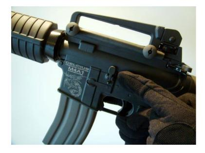
Just like the real M4/M16, 2 firing mode can be employed, semi –automatic and fully-automatic. After firing, always return the position to **SAFE**.
