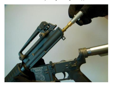
Occasionally lubricate the rubber seal and hop up unit from the loading port of the inner barrel. Use only 10% silicon oil, as many other lubricants such as mineral oil, automotive lubricants or WD-40 can immediately destroy the o-rings and other rubber components found within the inner barrel.
