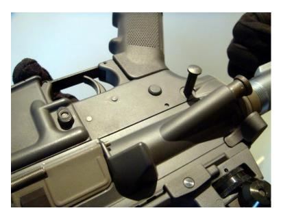
With your palm rested firmly on top of the stock, push the charging handle with your thumb to pivot the upper receiver. Please use considerably more force to open the upper receiver.
