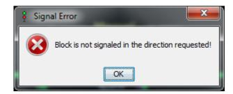
The track segment that is not signaled in the requested direction will flash for as long as this dialog is displayed. The dispatcher will not be able to do anything else in TSCAD until this error is acknowledged by pressing OK.
