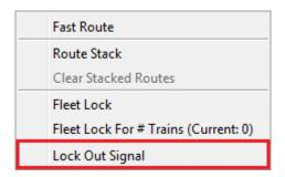
When doing so, a dialog will appear allowing the dispatcher to provide a reason for locking out the signal. This reason is optional, but recommended. The reason will be displayed to the dispatcher if he or she attempts to set up the signal without removing the lock out. Once the signal has been locked out, the color of the signal (head and mast) will change to purple.
