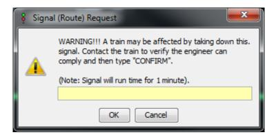
Once the signal is dropped, it will then "run time". During this timeout period, the dispatcher cannot align any other signals or switches in that OS.
