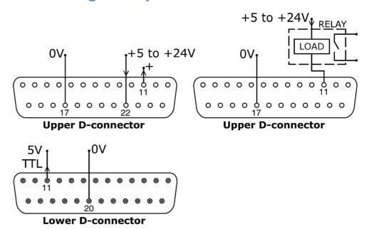
Output 2 is taken from pin 11 of the upper D-connector, depending on the logic state of the function assigned to Output 2. Alternatively, a load such as a relay coil may be connected to pin 11, ground to pin 17. Current will flow through the circuit depending on the logic state of the function assigned to Output 2. Do not connect to any device requiring more than 50mA.
