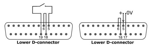
To enable remote direction control and disable the **DIRECTION** (**SHIFT, 1**) key on the keypad, link pins 6 and 18 of the lower D-connector. Connect a remote switch between pins 5 and 19 of the lower D-connector. Open switch for clockwise rotation,
