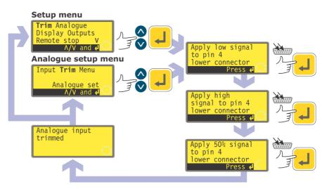
When the pump is under remote control, it tracks an analogue signal from the user's remote control system to pin 4 of the lower D-connector at the rear of the pump within the ranges 4-20mA, 0-10V or 1-5V. The **Trim** setup sequence allows the user to customise the process-signal-to-pump-speed calibration. The sequence may be entered directly from the Setup menu or from the Analogue setup menu.
