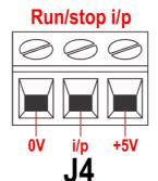
Remote run/stop: connect a remote switch between the  $\mathbf{i/p}$  terminal and the +5V terminal of the Run/stop i/p connector (J4). Alternatively a logic input may be applied to the  $\mathbf{i/p}$  terminal, ground to the  $\mathbf{0V}$  terminal. High input stops the pump, low input runs the pump. With no connection or with the switch open, the pump will default to running. To change or set the sense of the run/stop input, see 16.5 Remote stop in the Setup menu.
