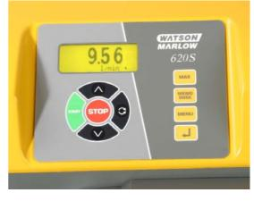
• START: starts the pump at the speed and in the direction shown on the dis-
