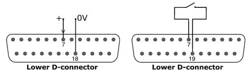
Remote run/stop: connect a remote switch between pins 7 and 19 of the lower D-connector. Alternatively a logic input may be applied to pin 7 of the lower D-connector, ground to pin 18. High input stops the pump, low input runs the pump. With no connection or with the switch open, the pump will default to running. To change or set the sense of the run/stop input, see 16.5 Remote stop in the Setup menu.
