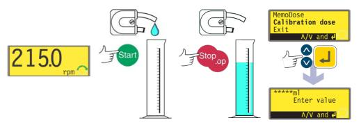
In the manual mode main screen, set the appropriate pump speed and direction using the UP or DOWN keys and the DIRECTION key. A slower speed may make it easier for the user to measure accurately - though it may not represent the duty condition.
