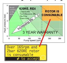
This pump's default running speed is 165rpm. It can be run at any speed up to 265rpm. Please note, however:
