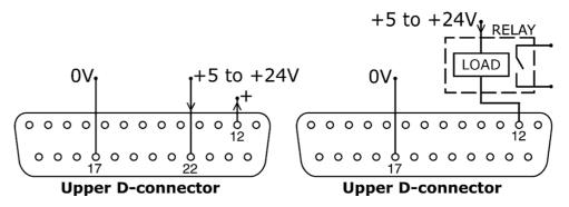
Output 4 is taken from pin 12 of the upper D-connector, depending on the logic state of the function assigned to Output 4. Alternatively, a load such as a relay coil may be connected to pin 12, ground to pin 17. Current will flow through the circuit depending on the logic state of the function assigned to Output 4. Do not connect to any device requiring more than 50mA.
