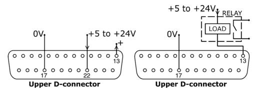
Output 3 is taken from pin 13 of the upper D-connector, depending on the logic state of the function assigned to Output 3. Alternatively, a load such as a relay coil may be connected to pin 13, ground to pin 17. Current will flow through the circuit depending on the logic state of the function assigned to Output 3. Do not connect to any device requiring more than 50mA.
