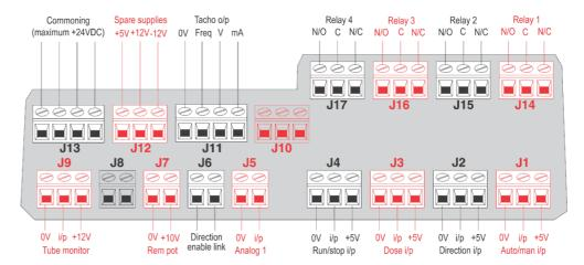
Never apply mains power to the terminals within the 620N module. Apply the correct signals to the terminals shown below. Limit signals to the maximum values shown. Do not apply voltage across other terminals. Permanent damage, not covered by warranty, may result. The maximum rating on the relay contacts of this pump is 30V DC; maximum load 30W. Note: Also suitable for low power: ie, 1mA at 5VDC minimum.
