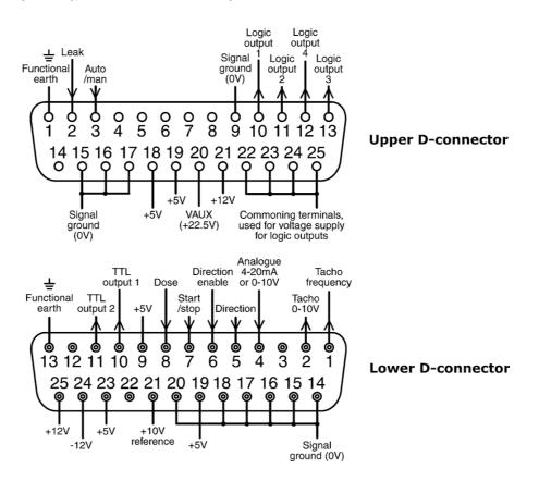
Recommended control cable: 7 strands 0.2mm, 24AWG, screened, circular, up to 25-core. The cable screen should be earthed either through the functional earth pin on the D-connector (pin 1 on the upper (male) 25-way D-connector) (pin 13 on the lower (female) 25-way D-connector), or through the metalwork of the socket or plug.
