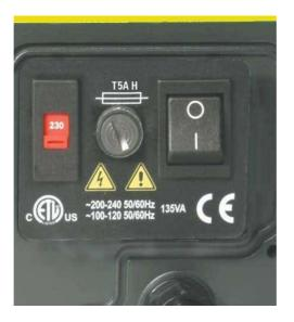
**Input line fusing**: type T5A H 250V 20mm time-delayed cartridge fuse, located in a fuseholder in the centre of the switchplate at the rear of the pump.
