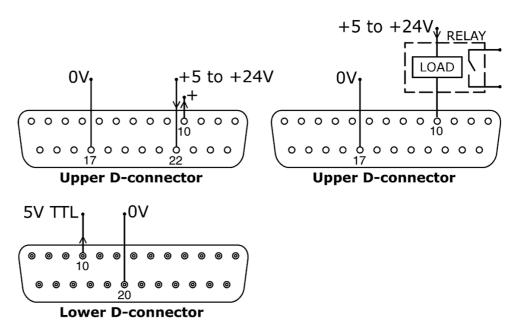
Output 1 is taken from pin 10 of the upper D-connector, depending on the logic state of the function assigned to Output 1. Alternatively, a load such as a relay coil may be connected to pin 10, ground to pin 17. Current will flow through the circuit depending on the logic state of the function assigned to Output 1. Do not connect
