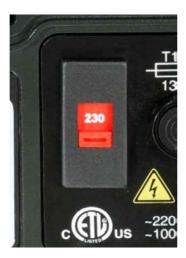
The voltage selector is mounted in the switchplate at the rear of the pump, protected from water by the 620N module (620DuN). The module must be removed to allow access to the switchplate. See 20.1 620N module removal and replacement. Set the voltage selector to 115V for 100-120V 50/60Hz supplies or 230V for 200-240V 50/60Hz supplies. Always check the voltage selector switch before connecting the mains supply. Make suitable connection to an earthed, single-phase mains electricity supply.
