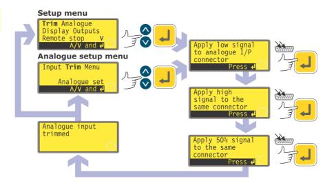
When the pump is under remote control, it tracks an analogue signal from the user's remote control system to the  $\mathbf{i/p}$  terminal of the Analogue 1 connectors at the rear of the pump within the ranges 4-20mA, 0-10V or 1-5V. The **Trim** setup sequence allows the user to customise the process-signal-to-pump-speed calibration. The sequence may be entered directly from the Setup menu or from the Analogue setup menu.
