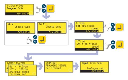
The pump displays a screen allowing you to set the speed for low signal input (4mA or 0V). Use the UP and DOWN keys to scroll the display to your chosen speed and press ENTER to confirm the figure.
