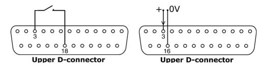
Connect a remote switch between pins 3 and 18 of the upper D-connector. Closed switch for automatic control; open switch for manual control. Alternatively a logic input may be applied to pin 3 of the upper D-connector, ground to pin 16. High input for automatic control; low input for manual control.
