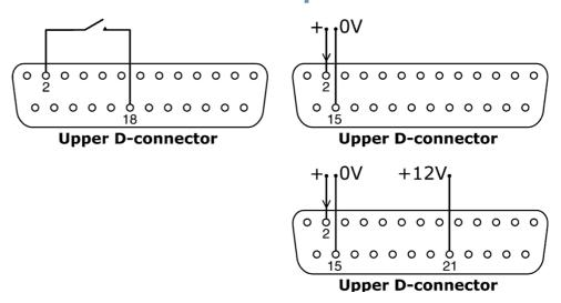
Connect a remote leak-detection device between pins 2 and 18 of the upper D-connector. Closed circuit indicates a leak. Alternatively a logic input may be applied to pin 2 of the upper D-connector, ground to pin 15. High input indicates a leak. Connect a Watson-Marlow leak detector in the same way, drawing 12V to power it from pin 21 of the upper D-connector.
