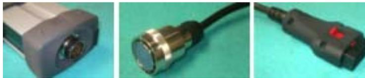
**Figure 27 MUX Fixed Male Large 55 Way Round Output Connector ↔ Free 55 Way Round Connector and Cable ↔ Free Male 16 Pin Plug (To Suit MB Connector X11/4 or OBD II)**
