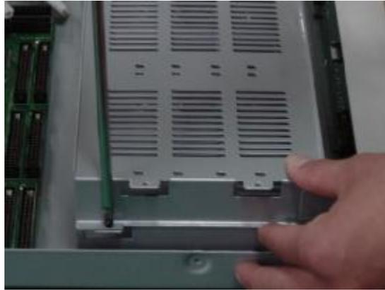
Figure 8 up part of HD bracket dismantle
