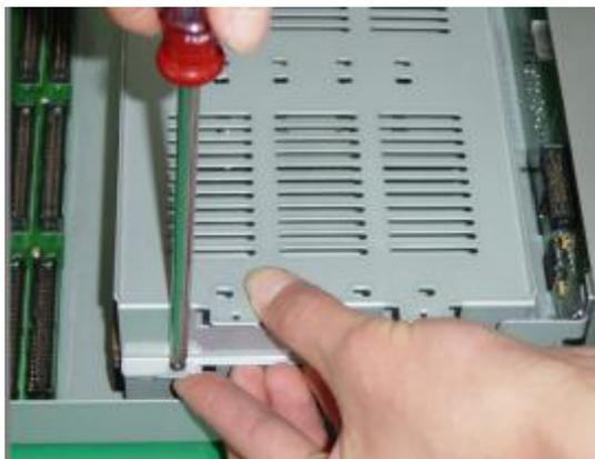
Figure11 Fix the HD Bracket
