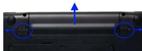
Insert the battery into the Netbook. Note that the battery is not fully charged. The battery should be left charging for about 12 hours. You are advised to make 3 such cycles fully discharging and fully charging the battery. This should help increase your battery life.
