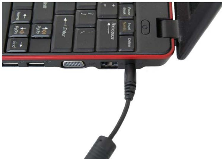
It is highly recommended to have the battery inserted when connecting your Netbook to the external power supply.
