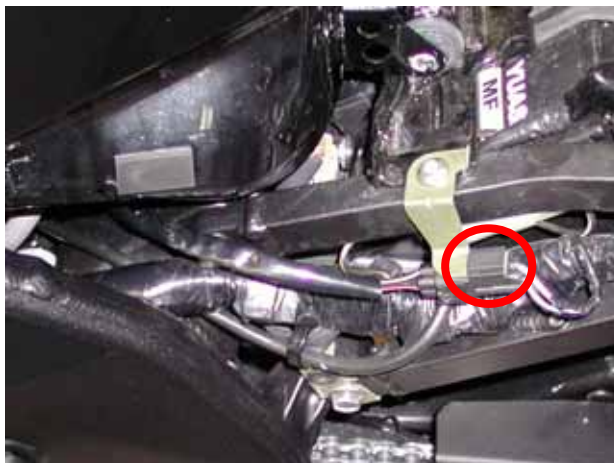
Figure 16: this black connector has to be removed
