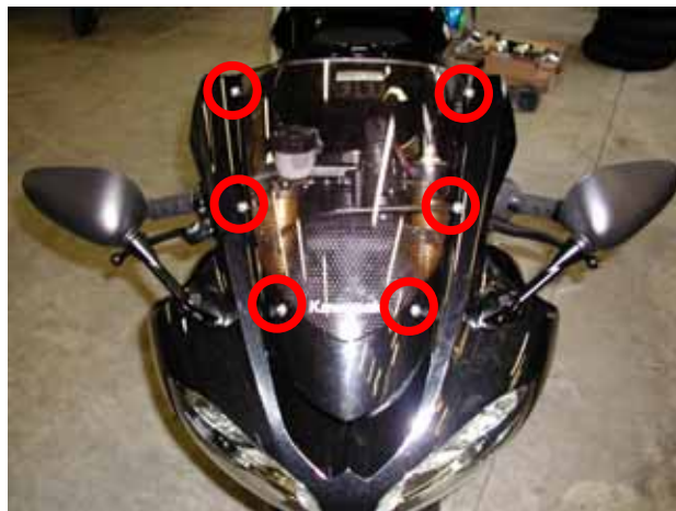
Figure 1: front transparent fairing – screws location
