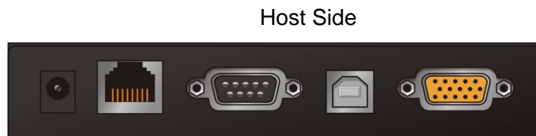
Figure 1-1. The connectors of single port IP-KVM switch host and console side
