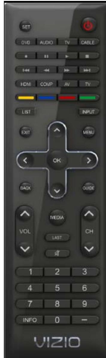
**BACK** — When use with the TV, this button behaves in the same way as the LAST button. It is used as a functional key on the set-top box for cable and satellite services with DVR features. It allows skipping back to previous prerecorded programs.
