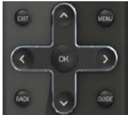
**Up (▲), Down (▼), Left (◀) or Right (▶) navigation buttons** — Press to navigate open menus, adjust other TV settings such as Brightness and Contrast, or turn menu options On and Off.
