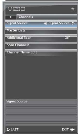
5. **Channel Name Edit:** If it is desired to change the name of the channel to a more comprehensive or favorite name, this option provides you with a choice. A small keyboard will be displayed and using the navigation keys, you rename the channel to your preference.
