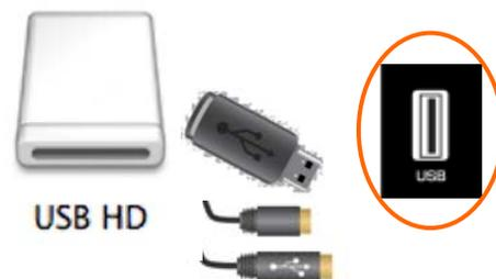
**Note:** This input is also used as factory service port. Please back up important files to prevent lost of data. Format your device to FAT32 and load your picture files, and enjoy your viewing. A high speed FAT32 storage device is also needed; preferable, new and memory emptied device for a better performance at least a 1Gb of memory device must be used.
