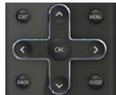
**Down (▼), Left (◀) or Right (▶) navigation buttons** — Press to navigate open menus, adjust other TV settings such as Brightness and Contrast, or turn menu options On and Off.
