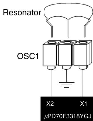
A 3-pin resonator with the capacitor can be inserted easily.
