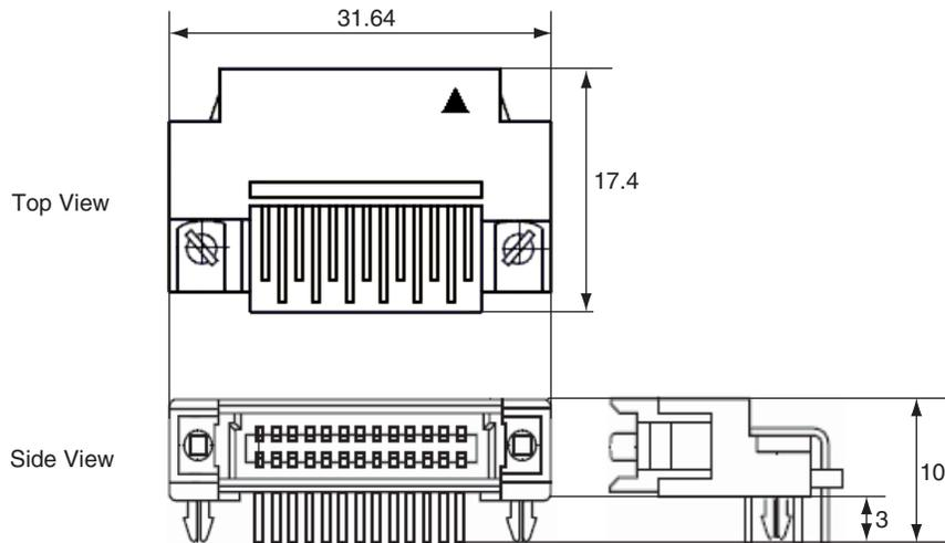
**Figure B-5. Mictor Connector (2-767004-2)**
