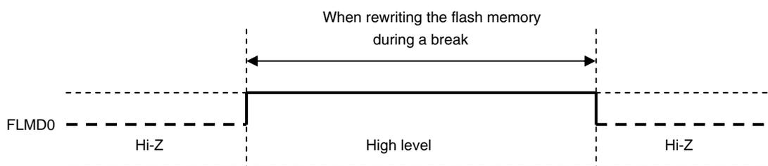
Handle the FLMD0 signal as shown in either (a) or (b) below. Whether the FLMD0 signal needs to be connected or not depends on the specifications of the target device.
