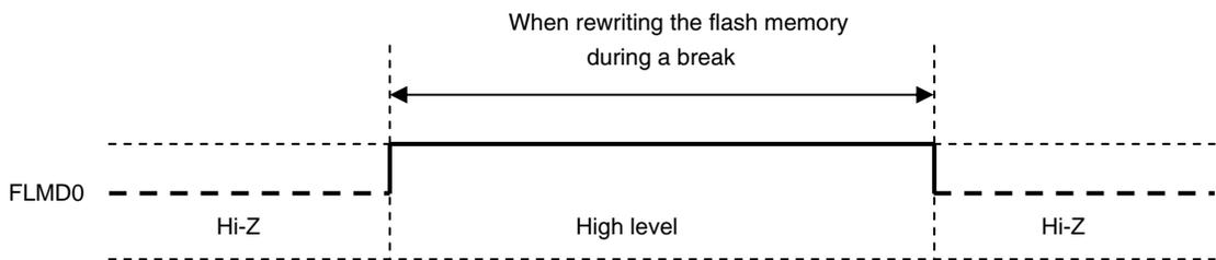
Handle the FLMD0 signal as shown in either (a) or (b) or (C) below. Whether the FLMD0 signal needs to be connected or not depends on the specifications of the target device.
