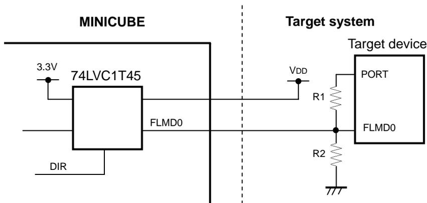
**Remark** The resistance of R2 must be at least 10 times the resistance of R1.
