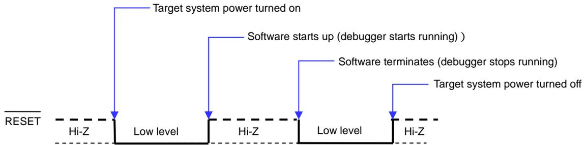
Connect the  $\overline{\text{RESET}}$  signal as shown in Figure 3-13 if any of the conditions listed below is satisfied. At this time, make sure that the  $\overline{\text{RESET}}$  signal does not conflict with the  $\overline{\text{RESET}}$  signal generated on the target system. When none of the following conditions are satisfied, leave open the pin for the  $\overline{\text{RESET}}$  signal that is output from the MINICUBE.
