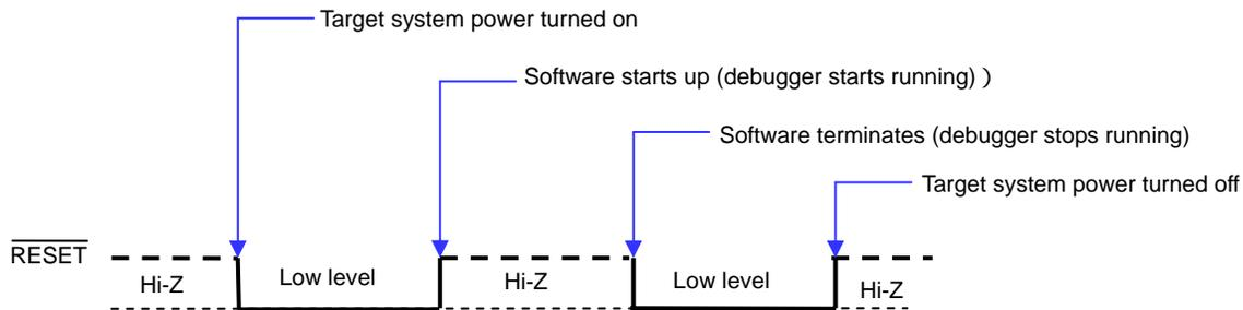
Figure 3-10.  $\overline{\text{RESET}}$  Pin Connection Example
