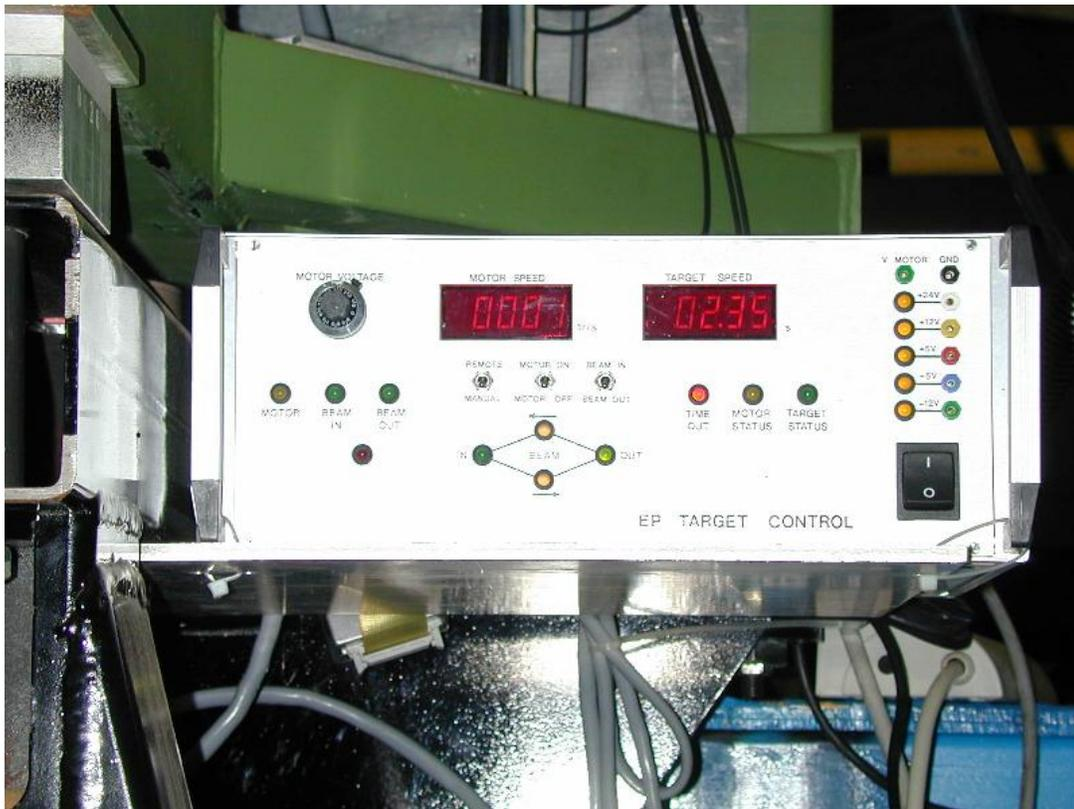
Figure 6.12: Control box for the eP target system.
