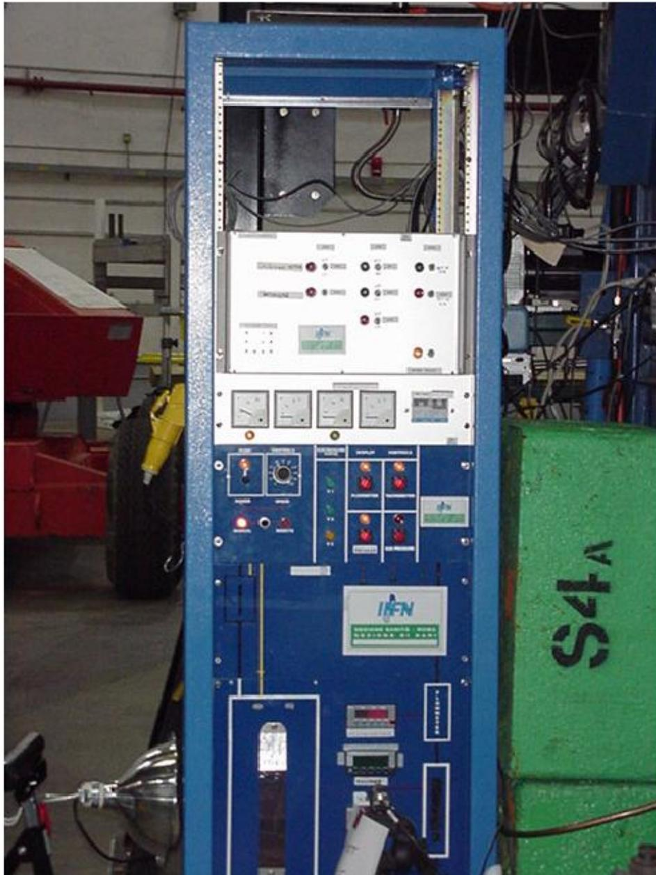
Figure 13.12: Waterfall target: control rack.
