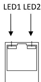
This LED lights up as orange and turns green when the encoder is powered on.
