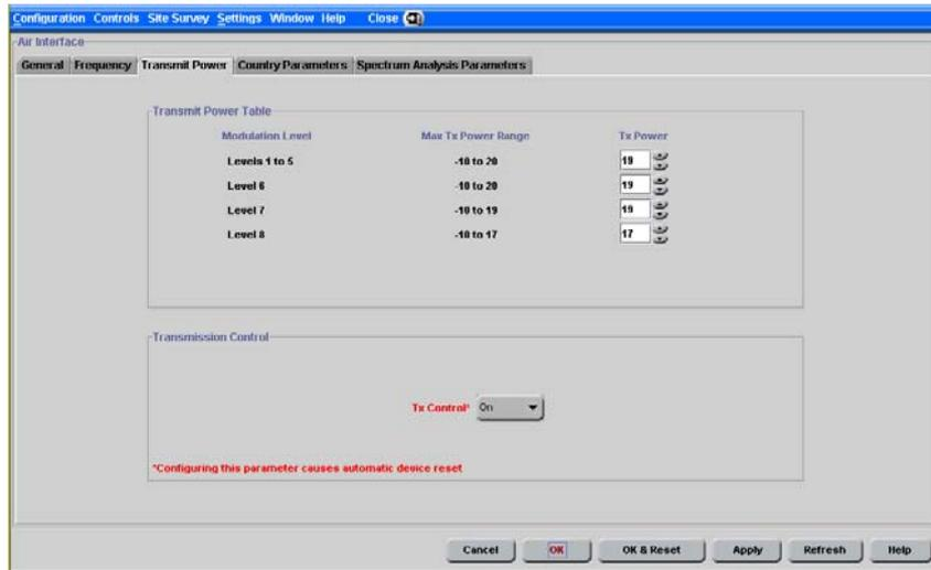
Figure 5-25: Air Interface Parameters Window - Transmit Power Tab - AU/BU
