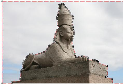
Masks are used in PhotoScan to specify the areas on the photos which can otherwise be confusing to the program or lead to incorrect reconstruction results. Masks can be applied at the following stages of processing:
