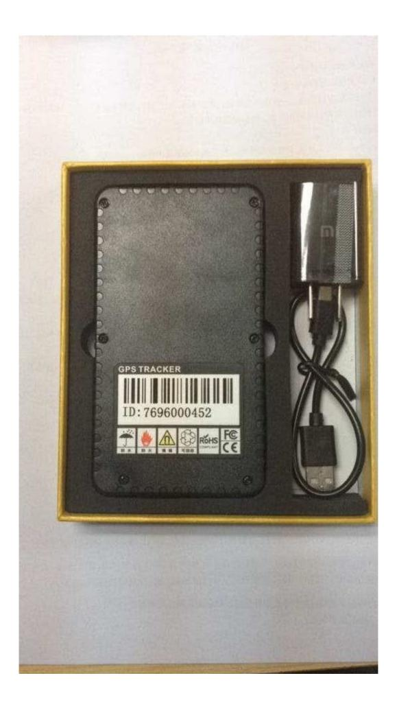
The AT-17 combined with the GSM and GPS technique and use the fireproofing material that arrived Industry standard which is 6PCS 18MM $\times$ 3MM super magnet and IPX-5, the internal battery is 8000MAH that can standby 100 days. The AT-17 can track the vehicle and person's position by SMS and GPRS on line tracking software.
