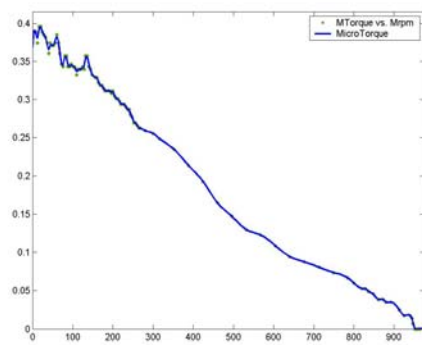
Fig. 13. Micro-Step mode Torque to rpm
