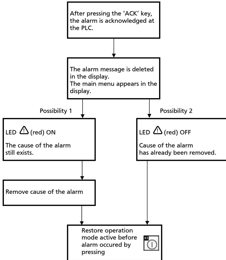
**Attention! It is not possible to restart the compressor as long as the cause of the alarm still exists!**
