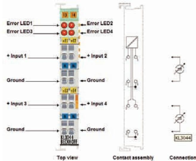
Figure 5.10: Analogue input terminals with 4 channels (4...20mA)
