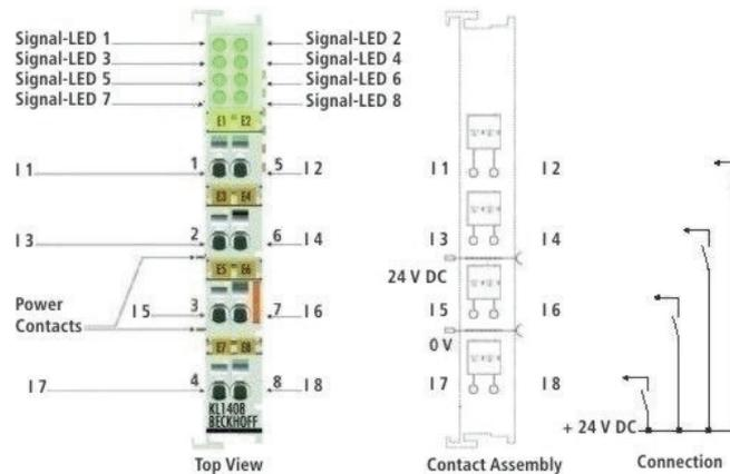
Figure 5.6: Digital input terminal with 8 channels
