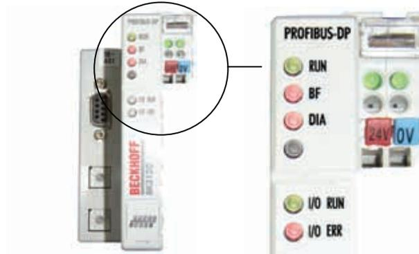
Figure 2: Periphery bus coupler with system LEDs
