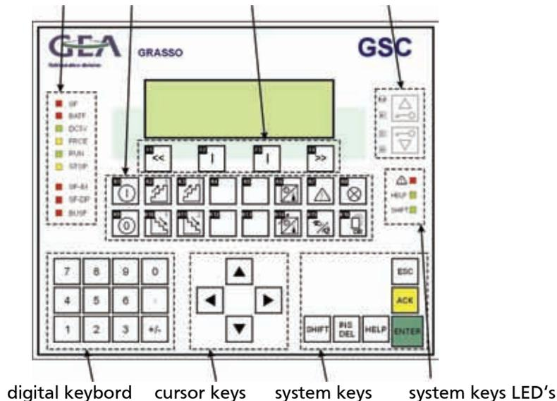
Figure 1.3: GSC operator terminal
