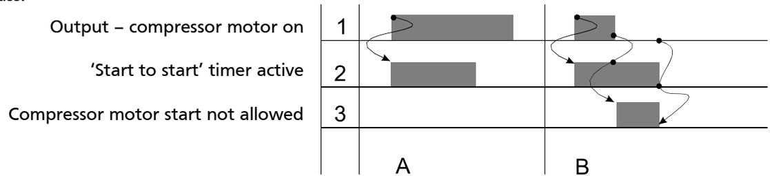
Case A: The compressor motor ran longer than the 'Start to start' timer, next start allowed immediately.
