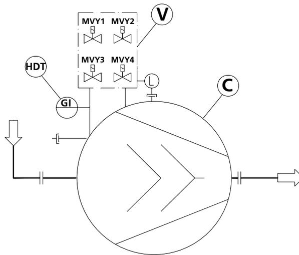
The solenoid valves for capacity adjustment are operated in pulses by the GSC control and are switched in pairs.
