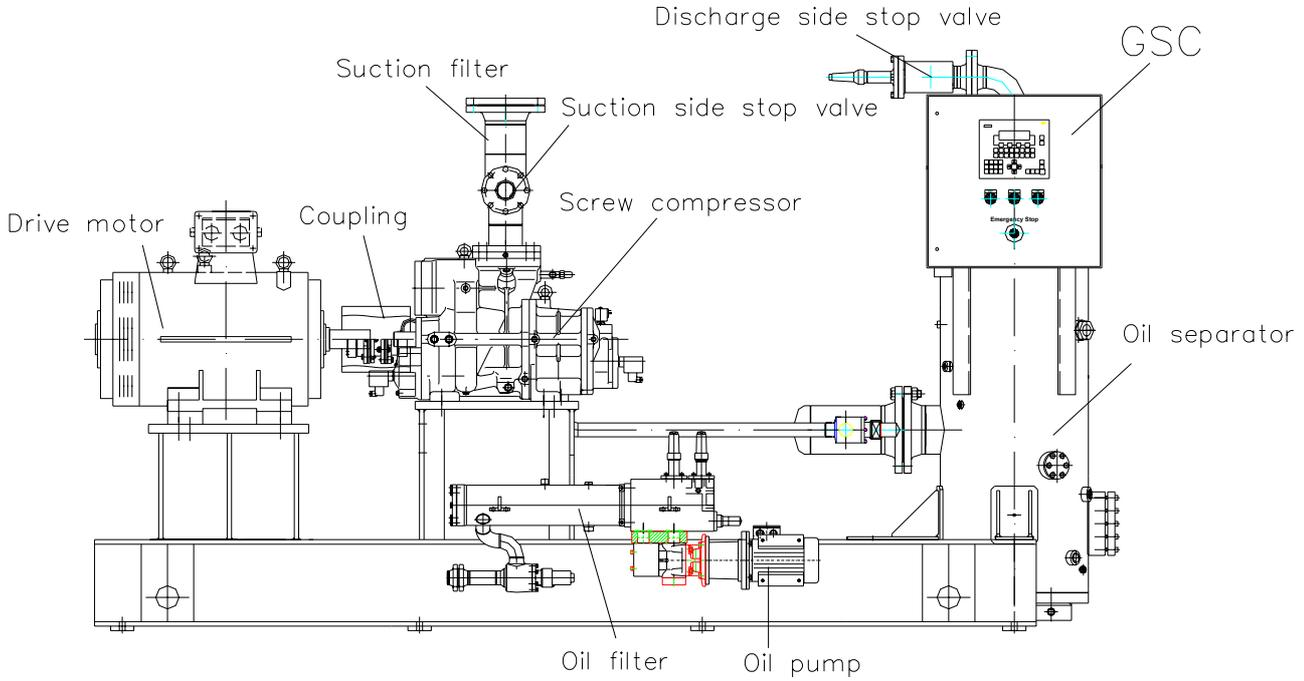
*Figure 0.1: View of screw compressor unit, type Grasso SP duo Medium*
