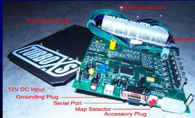
The UTEC allows you to control the main aspects of your car, Fuel, Timing and Boost. With the 4.1 firmware release the UTEC is looking more and more like a standalone ecu as it now contains it's own open loop fueling map. This is a nice features as your AFR's will be much more constant as your fueling with this mode enabled is based off a constant.
