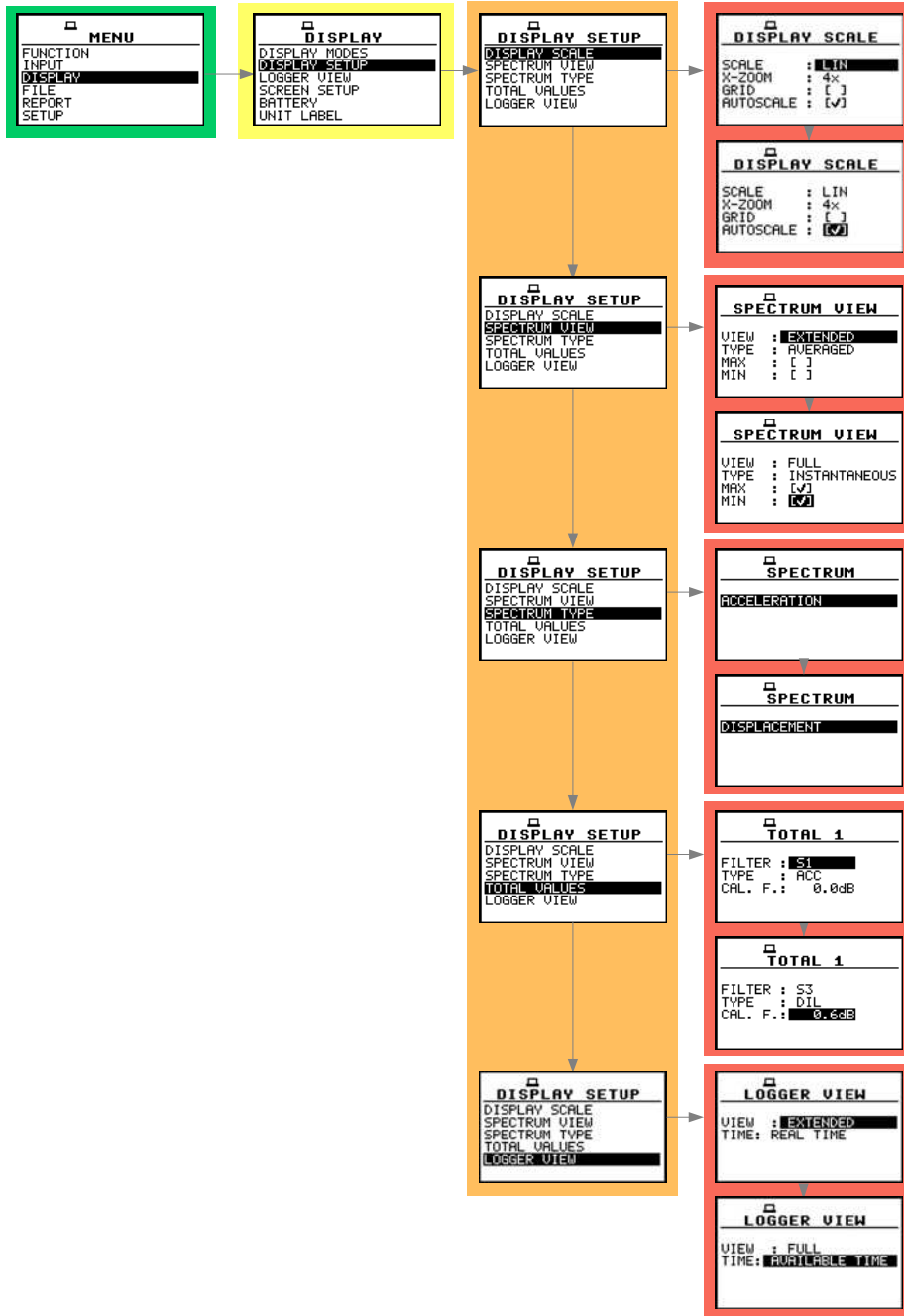
Control diagram of the DISPLAY SETUP sublist in 1/1 OCTAVE and 1/3 OCTAVE analysis of vibration
