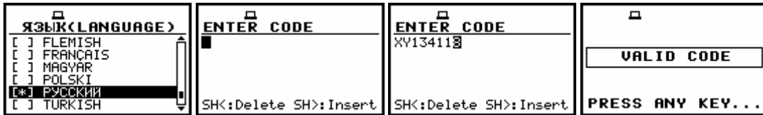
Displays during the entering of the access code to the Russian version of the user interface
