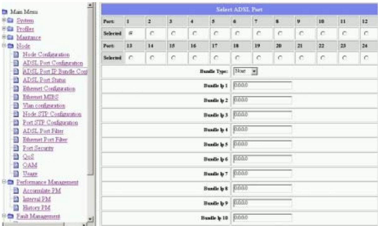
Figure 5-16 ADSL port bundle configuration
