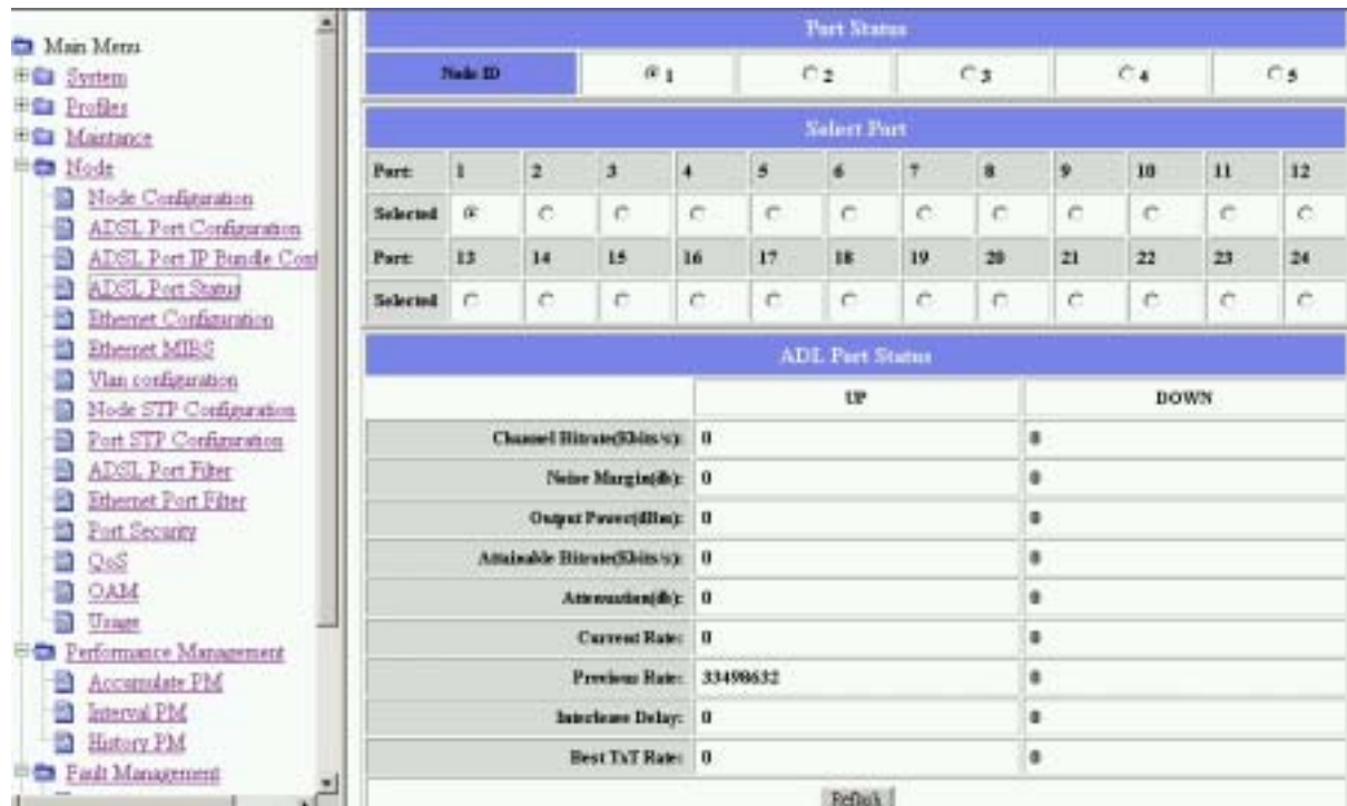
Figure 5-17 ADSL port status
