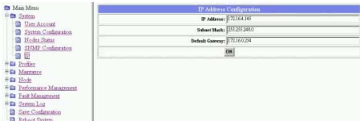
Figure 5-9 System IP configuration
