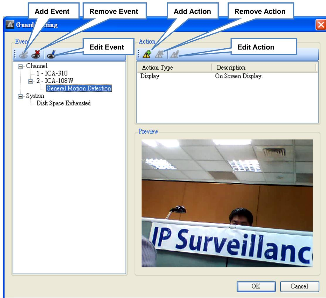
**Overview:** The Guard settings are to setup events and actions. For example, if you wish to have a certain channel to take action (such as Sound Alarm) when an event occurs (such as General Motion detected), you would set it up through here.
