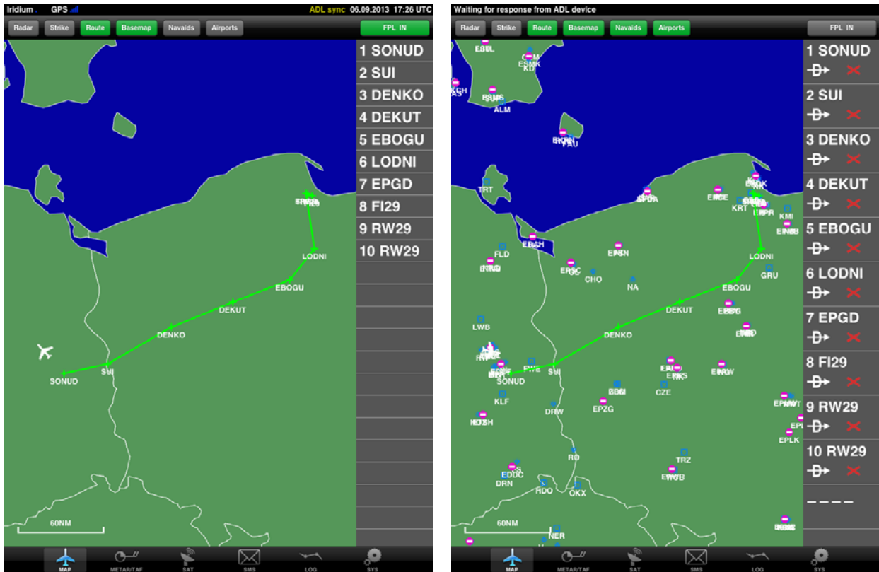
Figure 5 Flightplan: FPL IN activated vs. manual entry mode
