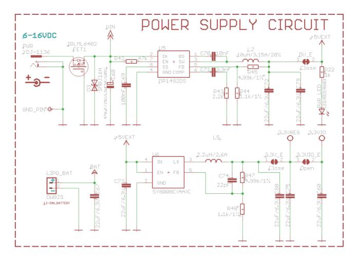
The jumper 5V\_E (5V Enable) which is closed by default enables powering the board via the power supply circuit.
