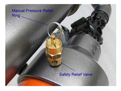
Safety Relief Valve will open automatically if pressure exceeds ~ 90 PSI Pull the ring for manual pressure discharge.
