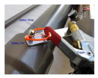
Trigger "Safety ON" position – trigger valve can not be depressed
