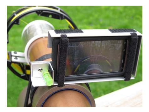
Augmented Reality Aiming Scope Mount (Custom made for specific Smart Phone models) The mount features a Soft Hood for an improved display contrast in bright ambient light and a Spirit Level Aid for quick field software calibration (0 degrees pitch)
