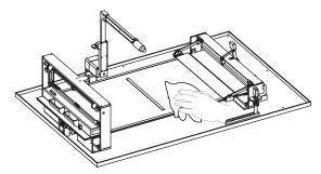
Avoid using water to clean BookDrive because it can damage the machine or cause electric shock. Make sure the machine is turned off and the plug is removed from the power outlet before attempting to clean.
