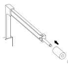
Insert the new roller into the page-turning arm.
