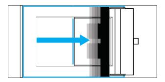
Adjust the length of the page-turning arm so that the roller is near but does not touch any part of the scanner platform.
