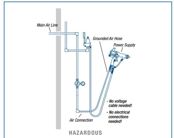
PRO Xs installation is quick and easy requiring very little time. Connect the grounded air hose to the air line and spray!
