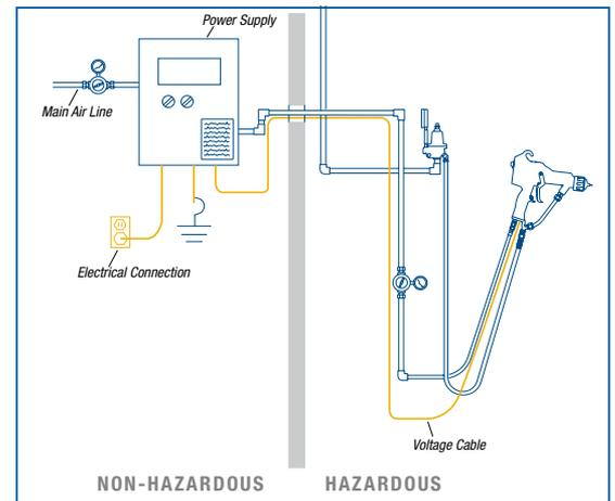
A typical competitors' installation requires a voltage cable that would run between the gun and the power supply located outside the hazardous area. Electrical connections are also required for complete installation.
