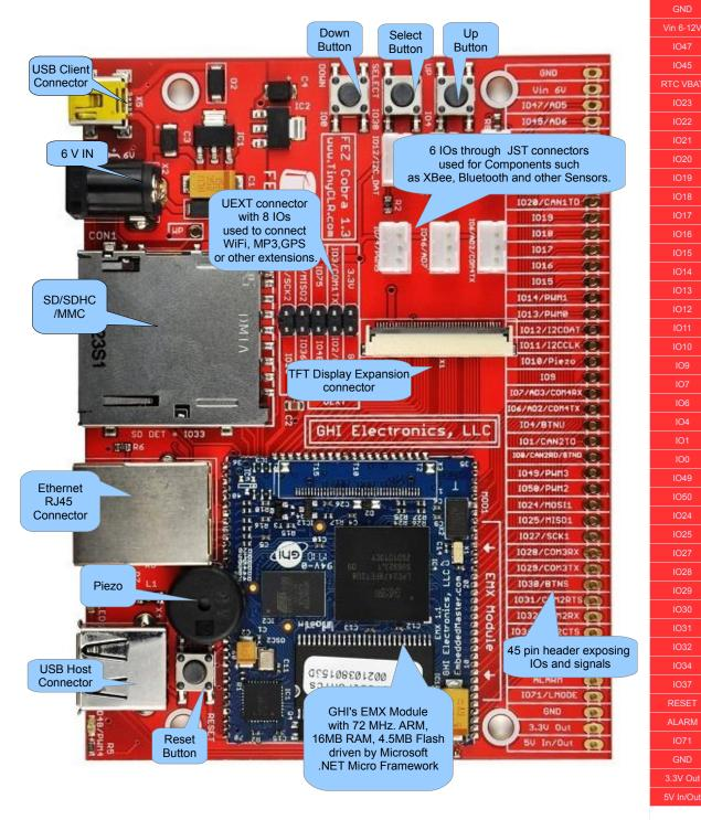
\* IO11 and IO12 are open drain pins with 2.2K pull up resistors.
