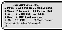
SAMPLES: 47 Number of samples/reading (1-65535) (47 rejects 60Hz, 57 rejects 50Hz) SAMPLES:
