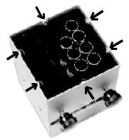
Remove the four screws hold ing the black module holding guide and remove the guide.
