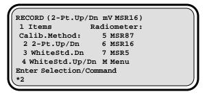
The presently configured Calib. Method and Radiometer is shown in parenthesis after RECORD. Select #2 for 2-Pt.Up/Dn and #6 for MSR16. Both of these must be configured before proceeding to the next step.
