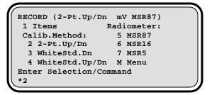
The presently configured Calib. Method and Radiometerisshown in parenthesis after RECORD. Select #2 for 2-Pt.Up/Dn and #5 for MSR87 or #7 for MSR5. Both of these must be configured before proceeding to the next step.
