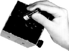
in a certain orientation so the pins mate properly with the module sockets. See the diagram on the following page. Orient the black stripe on the serial numbered module label towards the module socket.
