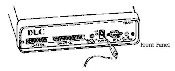
Connect the DLC to a personal computer or ASCII terminal using the appropriate RS232 cable. (If you are supplying your own cable, refer to appendix for cable wiring information).
