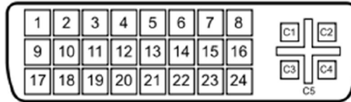
Pin Layout of the DVI-I connector (Dual-Link). (Female)
