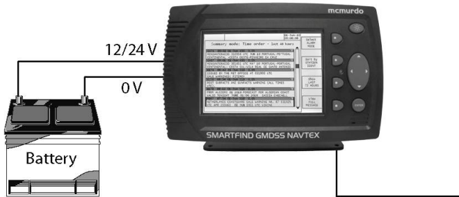
SMARTFIND GMDSS NAVTEX Minimum System
