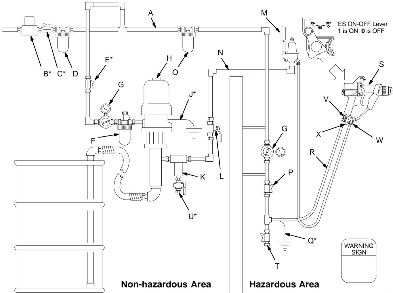
The air supply to the gun must be electrically interlocked with the ventilators to prevent the power supply from operating without ventilating fans on.
