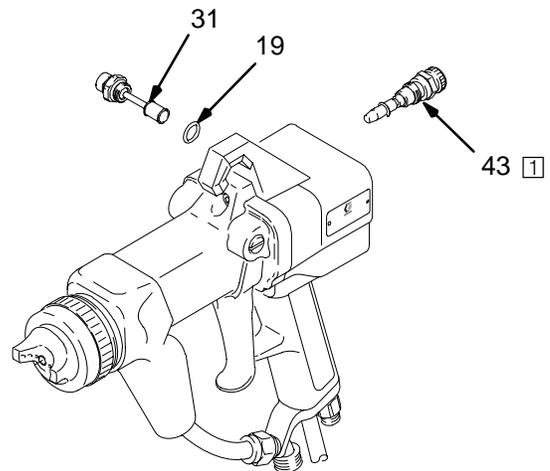
1 Apply PTFE paste to the valve housing threads (43d); Torque to 10–12 in-lb (1.1–1.4 N•m)
