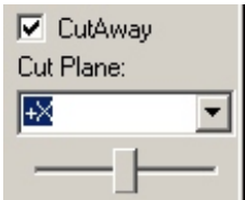
Figure 8.5: The cutting plane switch.
