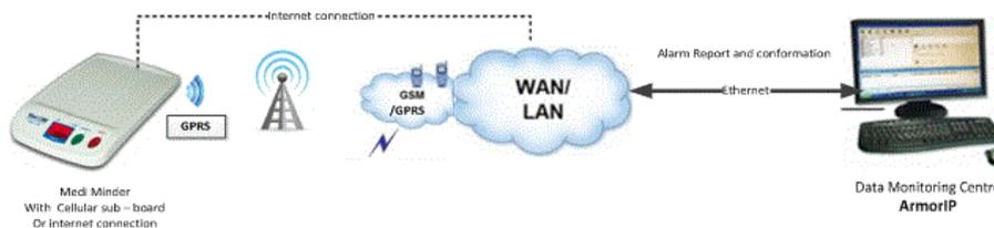
The Medi-Minder 3G unit has an internal GPRS/GSM Module to perform Network Reporting.
