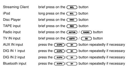
Once you have switched the **K2 Blu** to the desired source, you can listen to that source and also record the signal using the recorder outputs (TAPE OUT).
