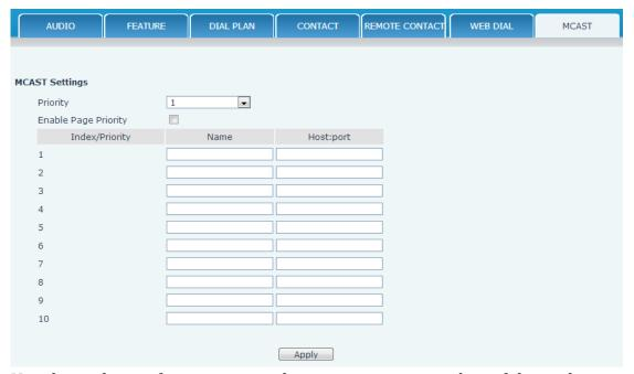
Use the multicast function to send notice to every member of the multicast is simple and easy. By setting the multicast key on your phone, you can send multicast RTP flow to the pre-configured multicast address. By listening multicast address is configured on the phone, listen and play the multicast address to send the RTP stream.
