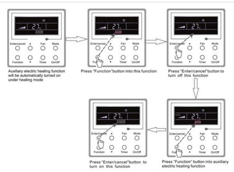
Fig.17 E-heater Setting
