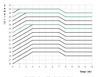
Fig.11 Sleep Curve of Sleep 2 in Cooling Mode
