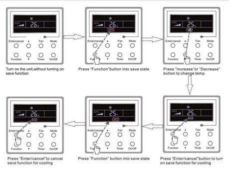
Fig. 15 Saving Setting for Cooling
