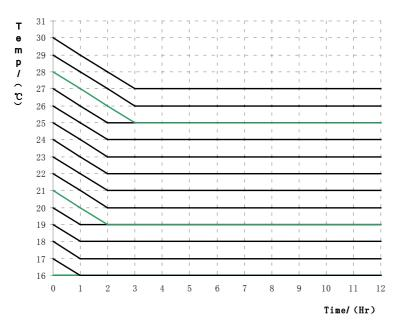
Fig.12 Sleep Curve of Sleep 2 in Heating Mode
