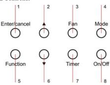
Fig. 3 Buttons on the Wired Controller
