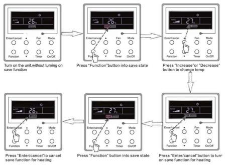
Fig.16 Save Setting for Heating
