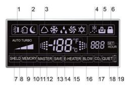
Fig.2 LCD of the Wired Controller
