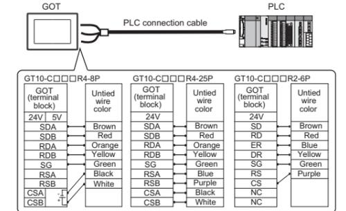
User-made cable is necessary, depending on the PLC. For the detail, refer to GOT1000 Series Connection Manual (Mitsubishi Products) for GT Works3.
