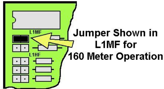
Figure 3 - Active Element L1MF Jumper Locations
