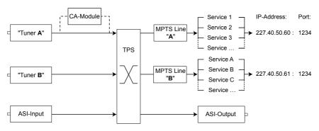
Additionally a transport stream is made available via the ASI output dependent on the signal path set.
