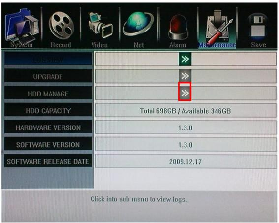
HDD information will display on the windows if DVR detection HDD correctly. Click [Formatting] to start HDD format.
