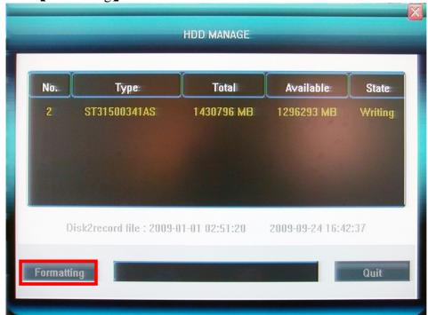
HDD information will display on the windows if DVR detection HDD correctly. Click [Formatting] to start HDD format
