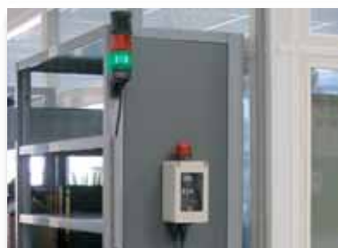
RadEye Area Monitor for neutron radiation
