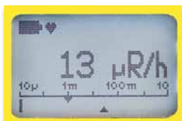
Background measurement Alarm thresholds - two triangles in the bargraph, indication low
