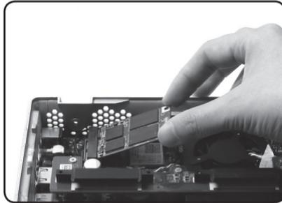
2. Gently press down on the mSATA SSD module and install the screw.
