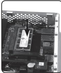
Note: This ZOTAC ZBOX accommodates two DDR3 SO-DIMM memory modules. You must install at least one module in one of the two slots.
