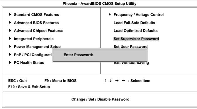
This option is for setting a password for entering BIOS Setup. When a password has been set, a password prompt will be displayed whenever BIOS Setup is run. This prevents an unauthorized person from changing any part of your system configuration.
